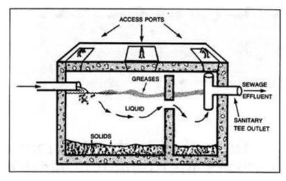
•Settlement and sedimentation takes place in the tank; increasing the amount of solid settlement reduces the amount of BOD that is carried out in the waste liquor.
